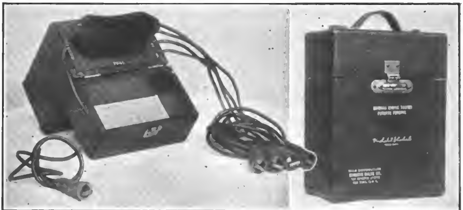
Fig. 1—Motor testing device brought out by the Dinshah company with which the cylinder conditions can be learned
